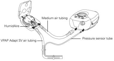
**3** Place the VPAP Adapt SV on top of the HumidAire. Never place the VPAP Adapt SV unit underneath the humidifier. (This is to avoid water spilling into the unit.)
